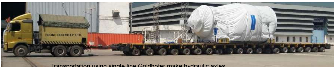
Transportation using single line Goldhofer make hydraulic axles
